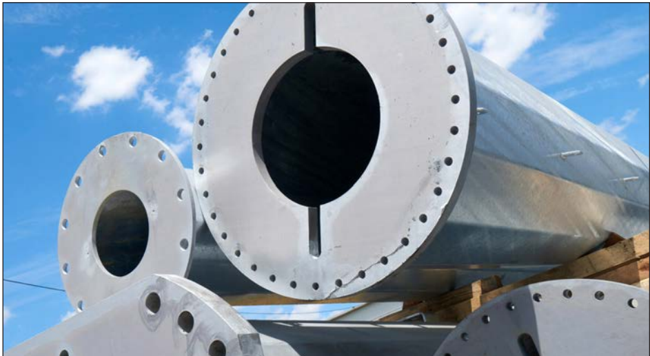
Nucor Corp., a North Carolina-based steel fabrication company, will launch a $204.5 million expansion project at its Brigham City plant in Box Elder County. The company's Towers & Structures unit will produce tapered tubular steel poles for high-voltage electricity transmission, like those shown in this Nucor company photograph.
