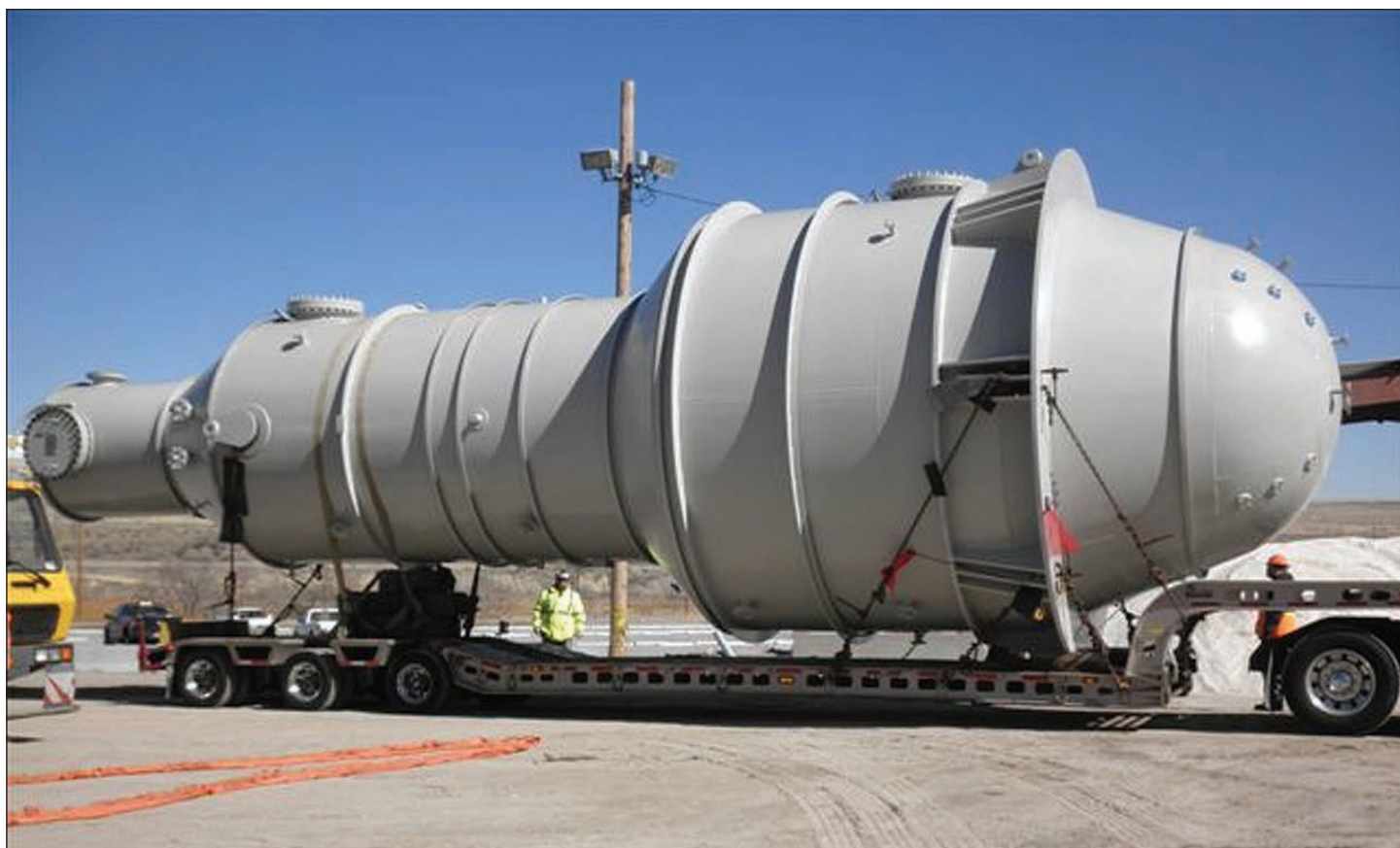
Kennecott's new crystallizer was manufactured offsite by Jacobs Engineering. Fifty-six feet long, its addition means construction at Kennecott's Molybdenum Autoclave Process facility in Magna is about 30 percent complete.
