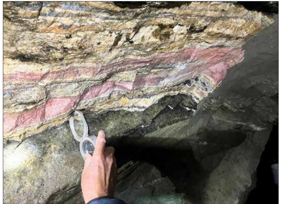
A vein of carbonite, the substrate that contains many rare earth minerals, is shown in this photo at the Sheep Creek deposit in Montana owned by Salt Lake City's U.S. Critical Materials. Ore from this mine will be processed at a pilot-scale plant to be developed by U.S. Critical Materials and Idaho National Laboratory. Photo courtesy U.S. Critical Materials Corp.
