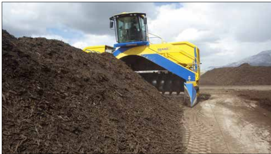
The Backhus A75 compost turner is used to turn the compost windrows. (Courtesy photos)
