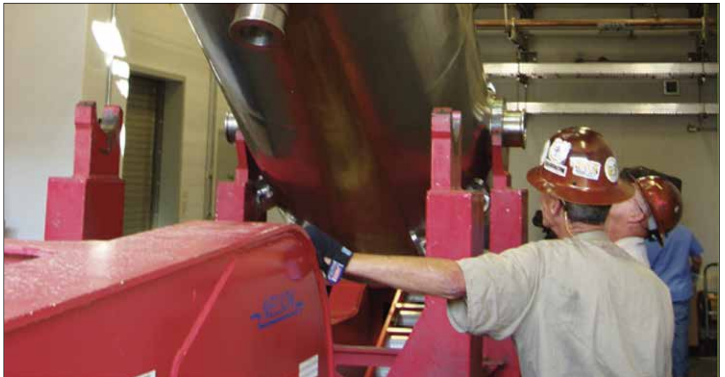
Crews at an EnergySolutions radioactive waste handling facility manipulate a cask designed for the transport of highly irradiated components from decommissioned nuclear power plants. The firm has been sold in a $2 billion transaction. (Courtesy EnergySolutions)
