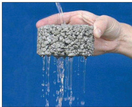
Pervious concrete allows precipitation to filter through into the earth rather than runoff into storm drains.
