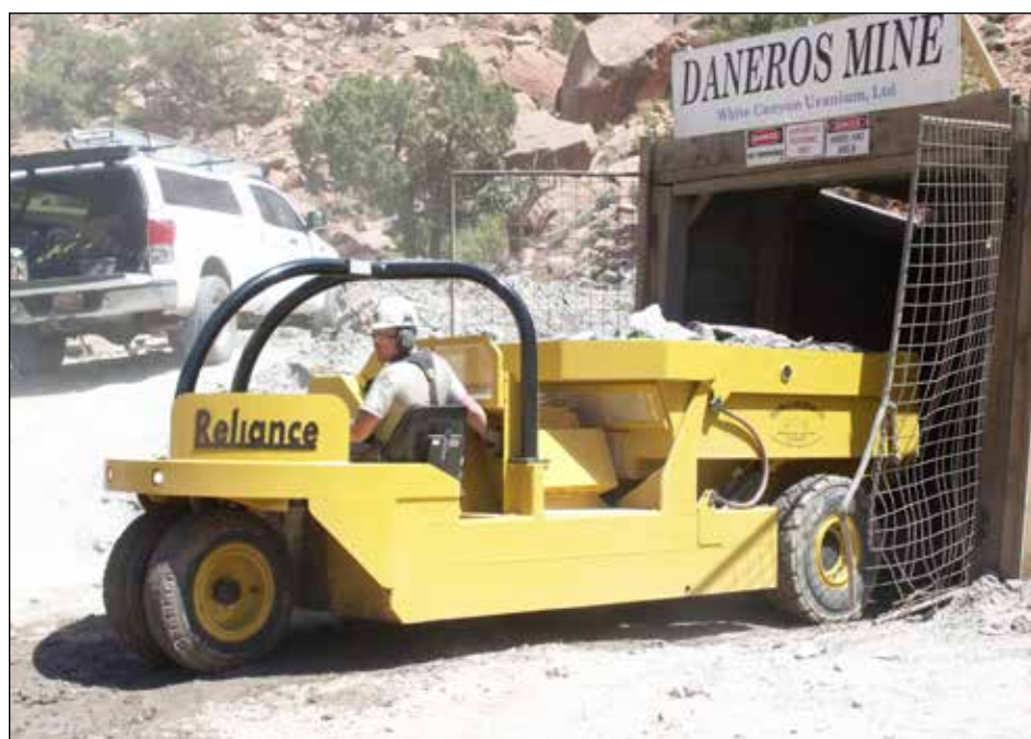
A Young's Machine Co. Series 960 dump truck exits a uranium mine in San Juan County. Anfield Energy has ordered eight similar trucks for its soon-to-be-opened Velvet-Wood Mine near Monticello. (Photo courtesy Young's Machine Co.)
